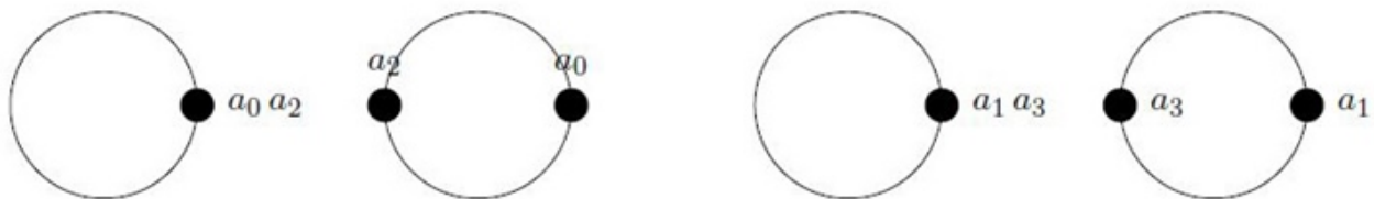
Figure 5. The first two terms are the discrete Fourier transform (DFT) of \{a_0, a_2\} and the last two are the DFT of \{a_1, a_3\} . Together they give the DFT of \{a_0, a_1, a_2, a_3\} , as shown in Figure 4.
